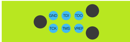
Figure 55: Foot print for tag-connect header
