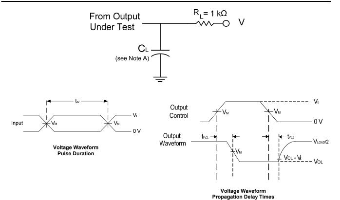
Notes: A. Includes test lead and test apparatus capacitance.
