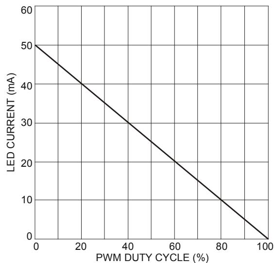
Fig. 17 Typical LED current response vs. PWM duty cycle for R_{EXT} = 13\Omega at 400Hz PWM frequency
