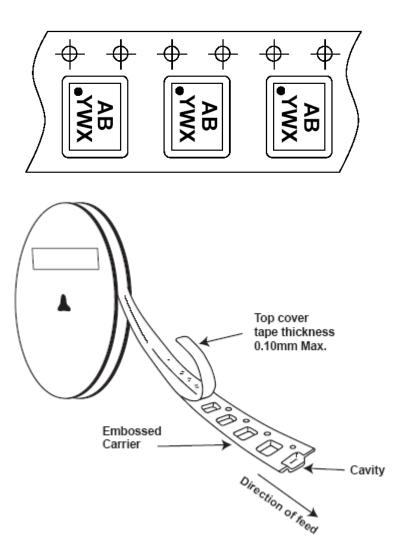
Note: 10. The taping orientation of the other package type can be found on our website at http://www.diodes.com/datasheets/ap02007.pdf.
