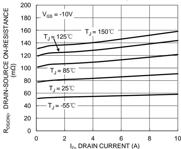
Figure 17. Typical On-Resistance vs. Drain Current and Temperature
