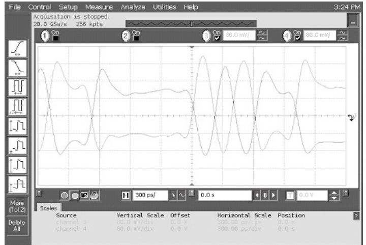
Data Waveforms, 2.5Gbps (left) & 5.0Gbps (right)
