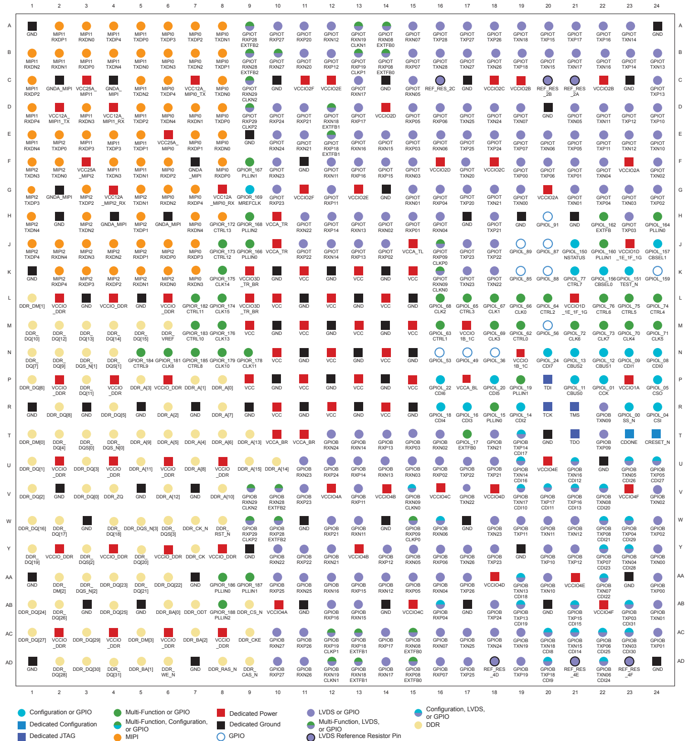
Figure 39: 576-Ball FBGA Pinout Diagram
